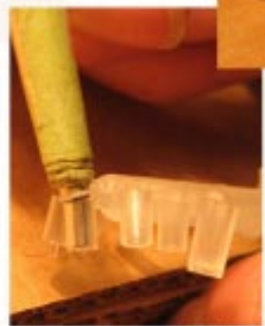
The magnet must be inserted into its plastic sleeve with the correct pole first using this fixture then inserted into the body.
