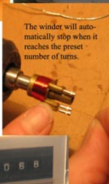
Move it left and right to keep the coil even.
