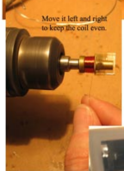
The winder will automatically stop when it reaches the preset number of turns.
