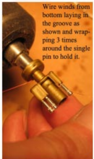
Wrap wire around as shown going on to the bottom from your thumb and forefinger.
