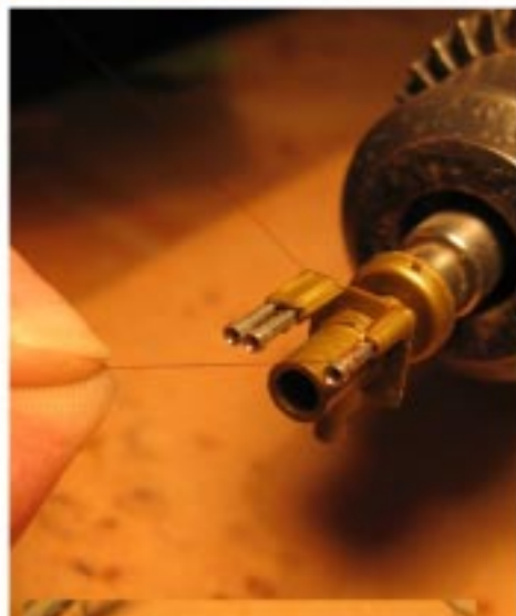
Move it left and right to keep the coil even.
